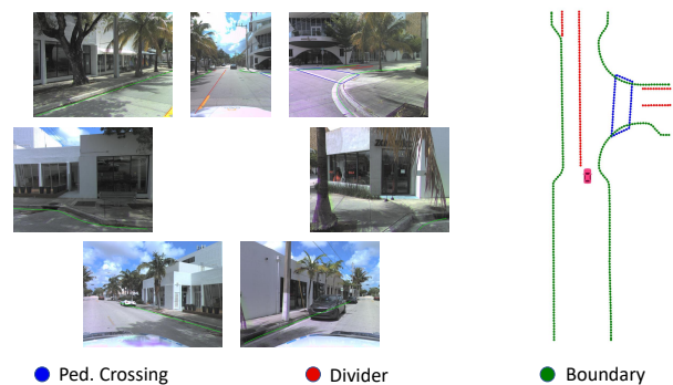
Figure 1. High-definition (HD) map is composed of instance-level vectorized representation of map elements (pedestrian crossing (blue), lane divider (red), road boundaries (green), etc.). Given inputs from onboard sensors (cameras), the goal is to construct the complete local HD map.
